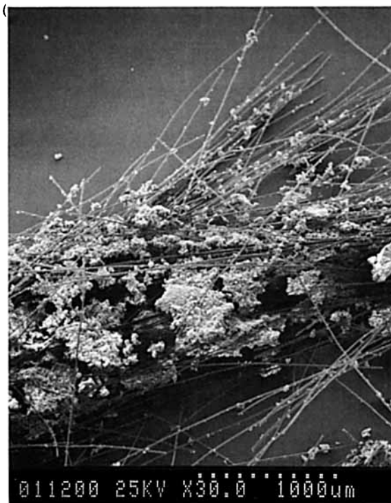
Figure 1 SEM pictures of the EVA-CF m -d before hot pressing: (a) EVA particles are deposited on carbon fibers (the emulsion method); (b) EVA particles agglomerate to a large extent among themselves (the solution method).
